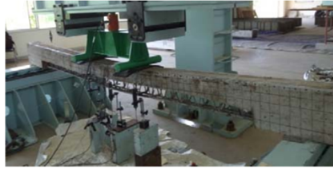
Fig. 6 Specimen Under Loading
