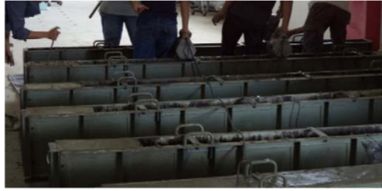
Fig. 3 Casting of Specimens
